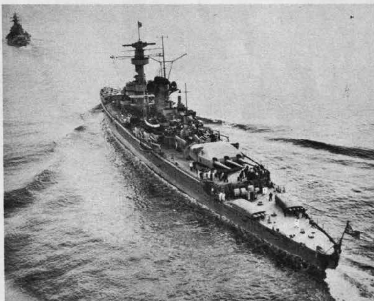
"Pocket Battleship" Lützow is really a cruiser with unusually heavy (11-in.) guns. It has the low, rakish outline broken by heavy pole foremast and single stack which characterizes German 11-in. gun heavies.
